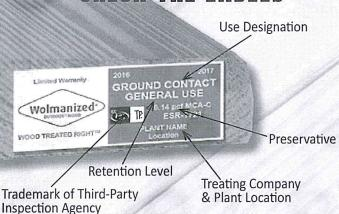
Always check the labels for the correct application; wood is treated with different loadings of preservative for different applications. Labels will designate Above Ground, Ground Contact or Ground Contact Heavy Duty applications, which refer to intended use. Check out the Homeowners/Literature & Resources section of www.WolmanizedWoodU.com to learn more. Reference to either AWPA U1 or ICC-ES ESR 1721 or ESR 1477 will indicate the product has been produced to accepted requirements and inspected.
